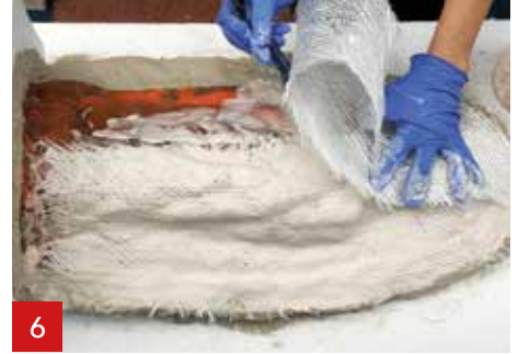
6 Add the A1 Triaxial fibre on the wet A1. Continue until the entire silicone mould is covered with A1 and a layer of A1 Triaxial fibre.
