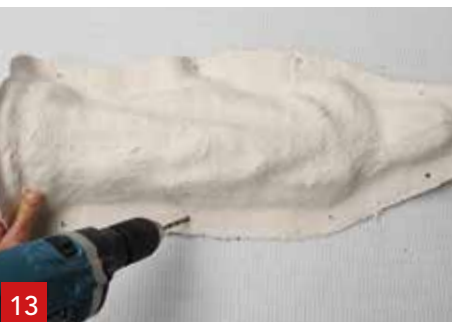
13 If needed, holes can be drilled in the A1 support mould to add bolts and nuts.
