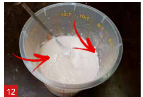
12 Stir the mixer till all lumps have disappeared ( \pm 1 min.) resulting in a smooth material.
