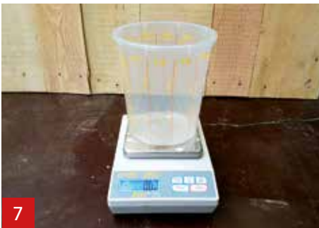
7 Place a cup on the scale. Calibrate the scale together with the cup (0.0 g).
