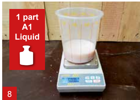
8 Weigh 1 part of A1 Liquid. In this example we use 500 g A1 Liquid.
