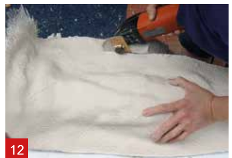
12 If desired, the A1 support mould can be finished with a multitool.
