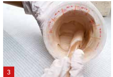
3 Mix the A1 Liquid, Thix A and A1 Powder resulting in a smooth material.
