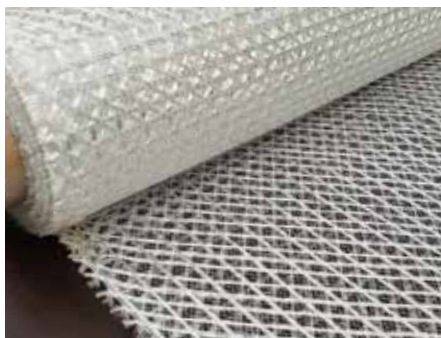
A1 Quadriaxial glass fibre 210 gr/m 2
