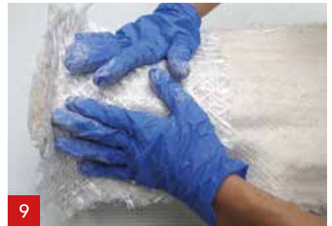
9 Press the A1 Triaxial fibre. The fibre can be formed/shaped well.
