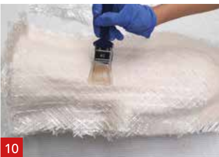
10 Brush this layer again with A1. Repeat until you have applied 4 layers of A1 Triaxial fibre.
