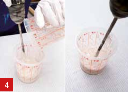
4 Gently add the A1 Powder to the A1 Liquid. Stir the mixer till all lumps have disappeared ( \pm 1 min.) resulting in a smooth material.
